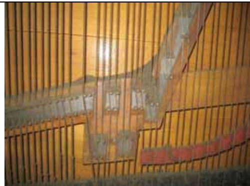
Stepped pinning of bridge
